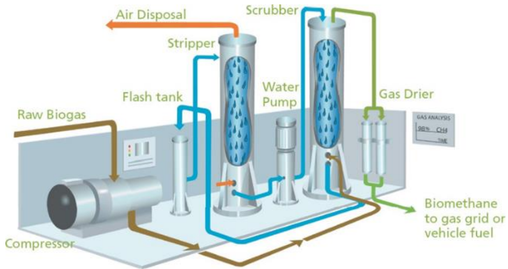
Figure 2. 6: Biogas Water Scrubber System Design. Illustration Credit: (Hudde, 2010)
